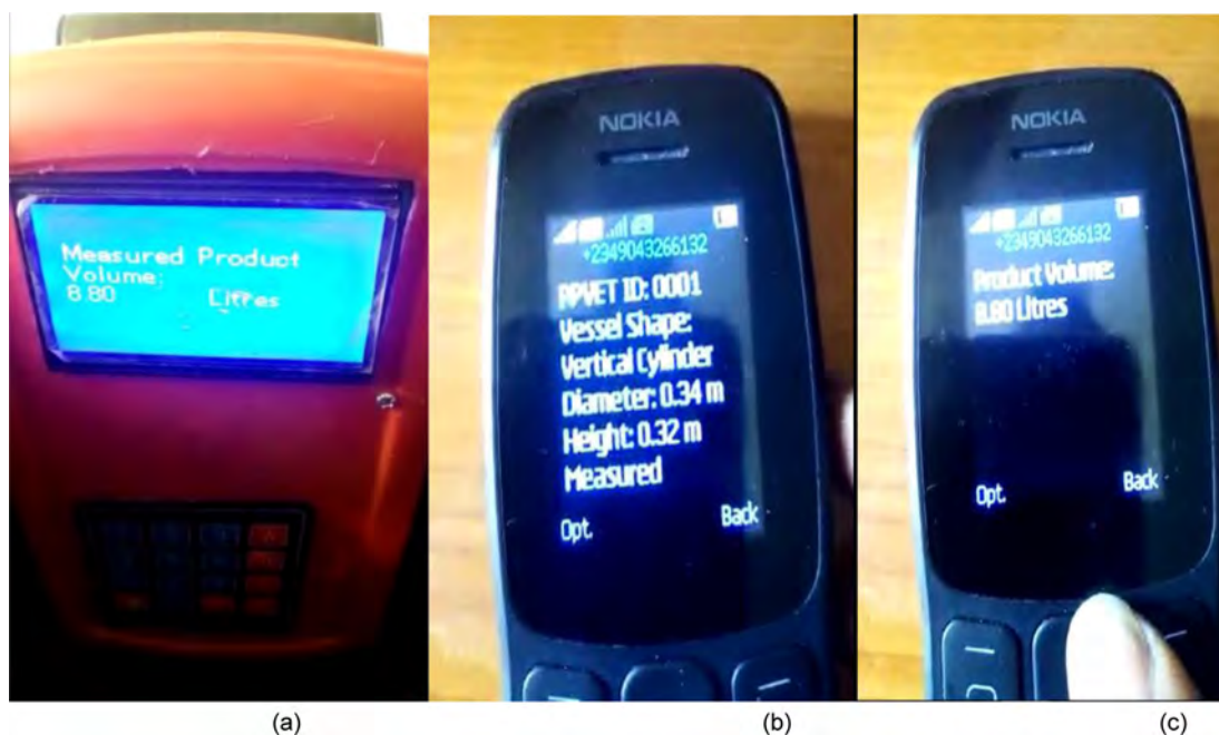
Figure 7—Automatic Volume Measurement by PPVET. (a) PPVET measuring 9L of Kerosene. PPVET sending Volume Alert message to authorized mobile number indicating PPVET ID, Vessel shape and size. (c) PPVET Volume Alert message to authorized mobile number indicating estimated volume of petroleum product (8.80 L).
