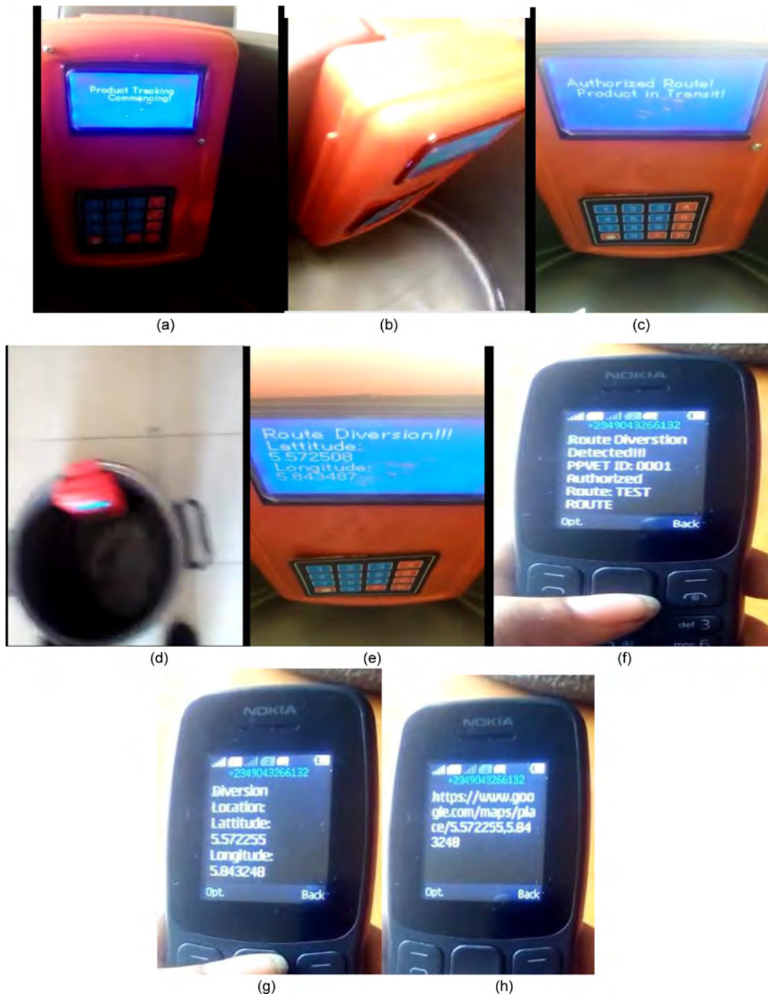
Figure 8—Product Tracking by PPVET. (a) Petroleum Product Volume Estimation by PPVET prior to product departure. (b) Petroleum Product being transported along authorized route (TEST ROUTE). (c) PPVET indicating petroleum product is within authorized route. (d) Petroleum Product being diverted from authorized route (TEST ROUTE). (e) PPVET successfully detecting product diversion within 30 seconds. (f) PPVET diversion text message sent to authorized mobile number showing PPVET ID and authorized route (g) PPVET diversion text message showing GPS location where diversion occurred. (h) PPVET diversion text message with link to google map pinpointing diversion location.
