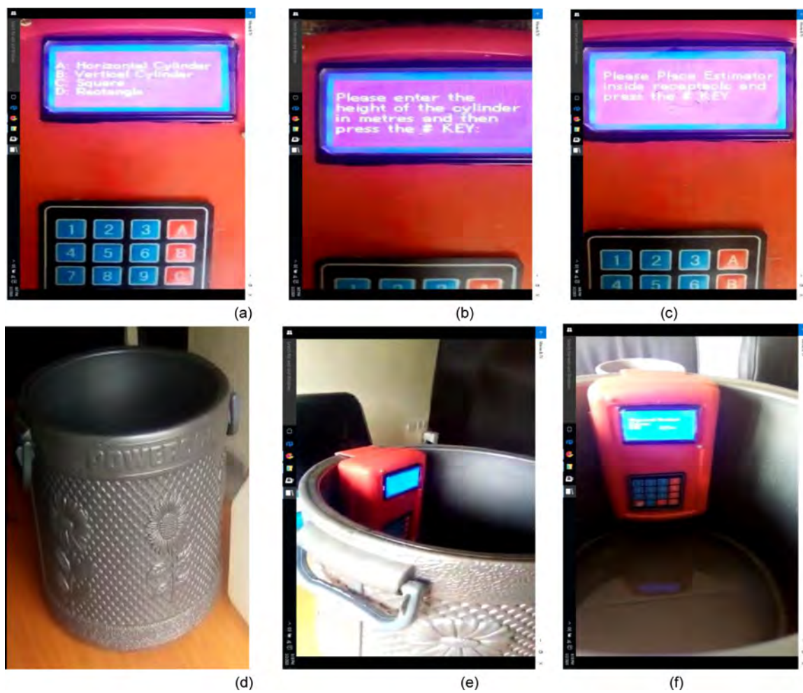
Figure 6—PPVET (a) Unit requesting user to select shape of receptacle. (b) Unit requesting user to input height of receptacle in metres. (c) Unit requesting user to mount estimator on receptacle for volume measurement. (d) Vertical cylinder with 0.34 m inner diameter and 0.32 m height used for PPVET volume measurement tests. (e) PPVET mounted on vertical cylinder containing petroleum product. (f) PPVET conducting automated volume measurement and estimation of petroleum product.
