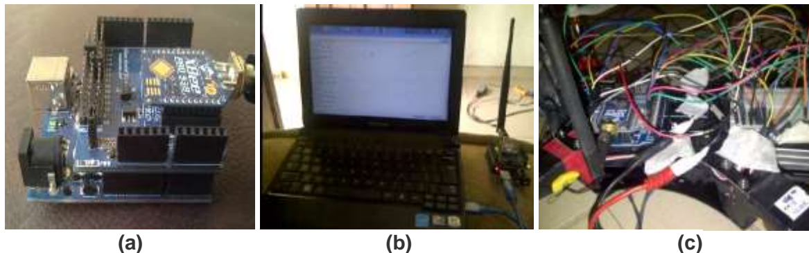
Fig. 2. (a) Xbee Pro 900HP on Xbee Shield stacked on Arduino Uno. (b) First Xbee connected to host PC at remote station. (c) Second Xbee mounted in AROSS system.
