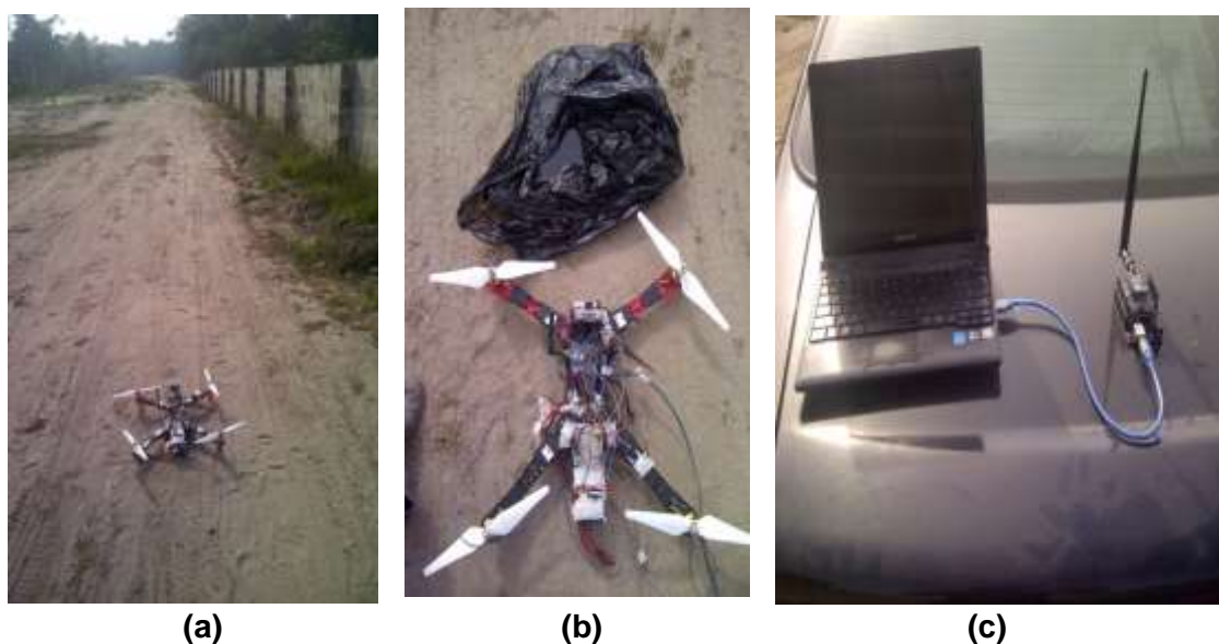
Fig. 6. (a) AROSS system patrolling 100 pipeline surveillance route. (b) AROSS system detecting presence of 1 liter crude oil spill along surveillance route. (c) Host PC at remote base station 100 m away from surveillance route.
