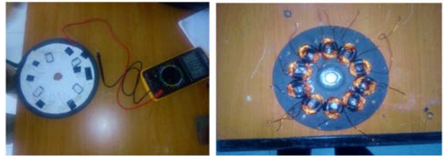
Figure 4. Stator coil (testing and construction).
