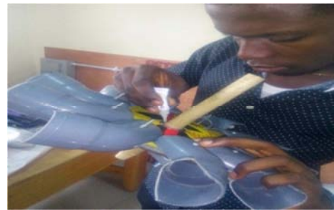
Figure 10. Fixing of shaft to the turbine wheel.
