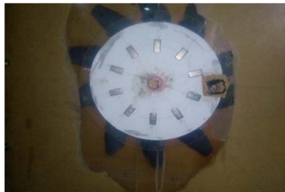
Figure 5. Rotor (N50 Neodymium magnet).
