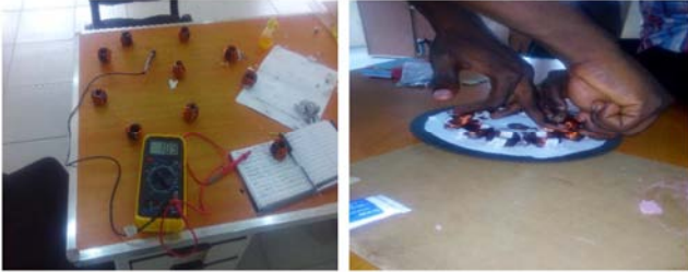
Figure 7. Winding the Alternator coils.
